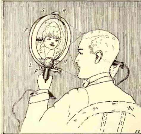
What the Future Telephot Will Look Like in Order to be Practical. Light R Throws Light on Speaker's Face and is Reflected into Lens L. Instead of a Mouthpiece, the Mikes, H of the Sensitive Transmitter Inside. Frame F Pick Up the Speech. The Picture of the Distant Person Appears on Screen S.
